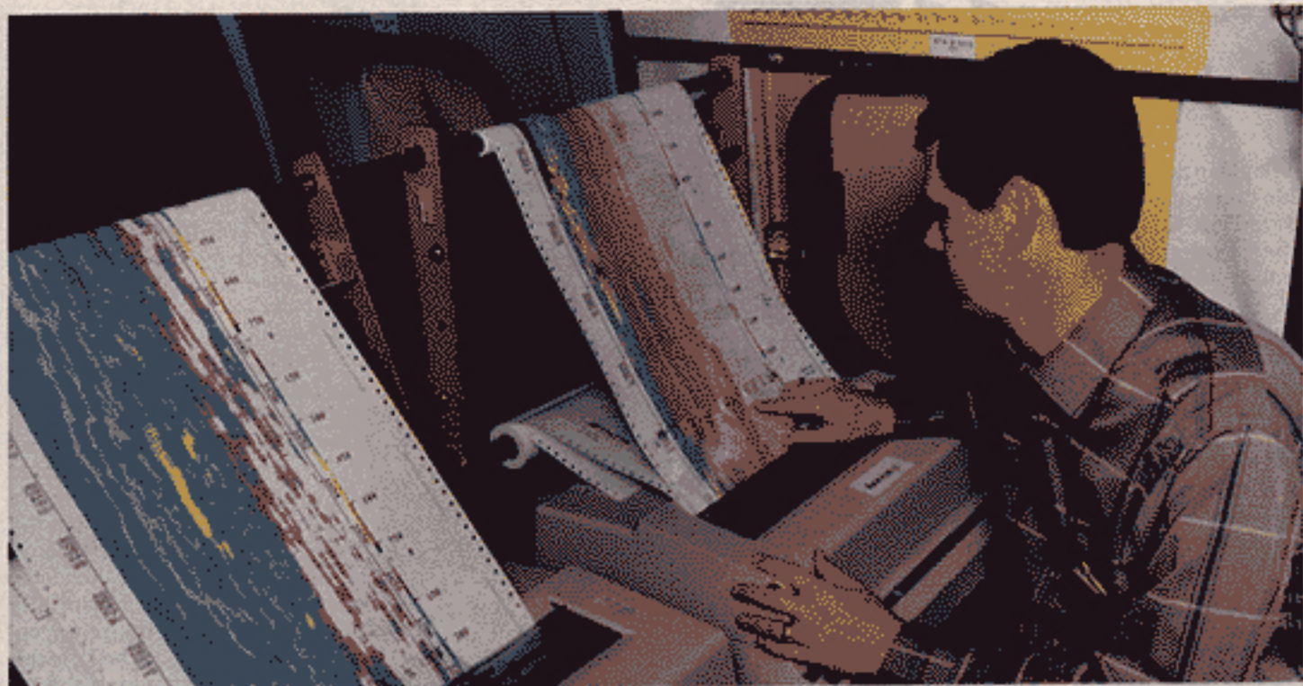
NASA Langley Research Center scientist Edward V. Browell monitors the plotter readout of his "ozone and aerosol differential absorption laser detection and ranging system" experiment. The experiment uses laser beams to analyze the atmospheric chemistry overhead a DC-8 by measuring
